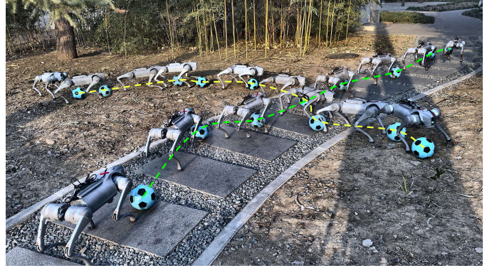
Fig. 1. Experiments on dynamic ball dribbling over rugged terrains. The green trajectory traces downhill dribbling over stone slabs and loose gravel; the yellow trajectory shows dribbling across a mixed surface of wet mud, raised curbs, stone slabs, and loose gravel.
